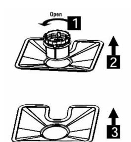
Step1: Rotate the fine filter counter-clockwise;
